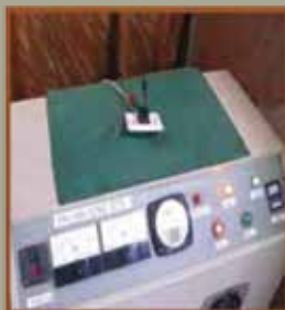
Switch - high voltage test
