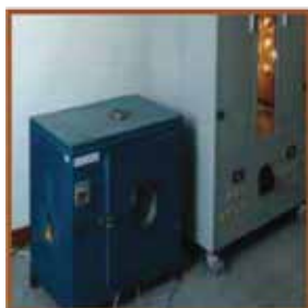
Dimmer regulator - life test
