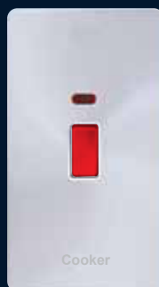
MT5221: 45A, double pole switch, red rocker, marked "Cooker" with neon, 2 gang
