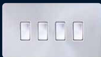
MT5207: 10AX, 2 way switch, single pole, double plate, 4 gang MT5208: 20AX, 2 way switch single pole, double plate, 4 gang
