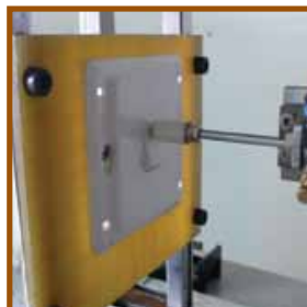
Switch - normal operation test
