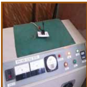
Switch - high voltage test
