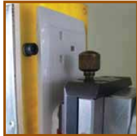
Socket - normal operation test
