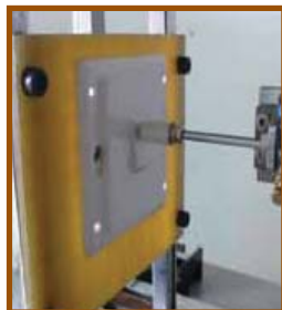
Switch - normal operation test
